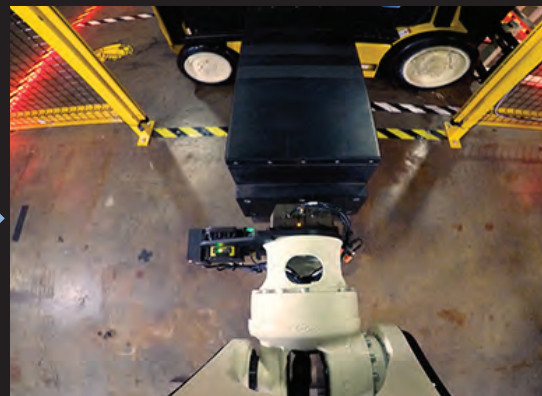
SENSORS ENABLE ARM TO POSITION ITSELF IN FRONT OF BATTERY CRADLE
