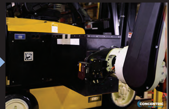
ARM INSERTS BATTERY INTO FORKLIFT
