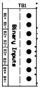
The terminal connections are labeled along the edge of the Auxiliary I/O Board next to terminal block (A4-TB1). Each binary input is optically isolated and has a polarized pair of terminals. Observe the pos(+) and neg(-) designators when wiring the terminal block.
