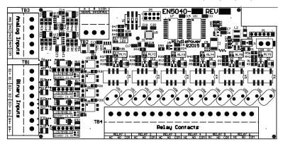
For component details of the Auxiliary I/O Board (A4), refer to standard drawing:
