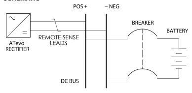
To wire ATevo for remote sensing, install twisted-pair cabling from the remote sense terminals to the battery terminals or dc bus. ATevo control circuitry measures dc voltage at the battery terminals and controls charger output to maintain battery voltage at the desired float or equalize voltage.
