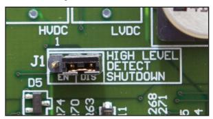
The High Voltage Shutdown jumper (J1) is located center-right, on the Main Control Board (A1).
