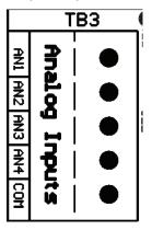
Terminal connections are labeled along the edge of the Auxiliary I/O Board next to terminal block (A4-TB3). The analog inputs are **NOT** isolated, and must be referenced to the negative (-) dc bus.
